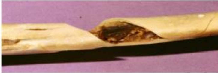
Figure 16.6 Failure in torsion of a circular bar of brittle cast iron, showing a tendency to tensile fracture across a helix on the surface of the specimen.
